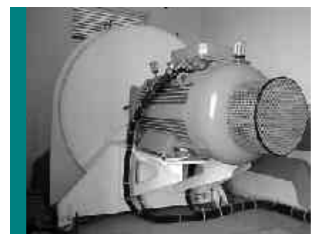
Fig 2: Flywheel and synchronous machine.
